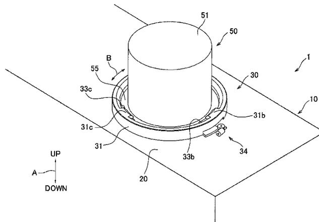
move the second restricting portion **33a** along an extending direction B between a first position, in which the second restricting portion **33a** is opposed to the flange **55** of the container **50** in an up-down direction A, and a second position, in which the second restricting portion **33a** is opposed to the recessed portion **56a** in the up-down direction A without being opposed to the flange **55** in the up-down direction A.
