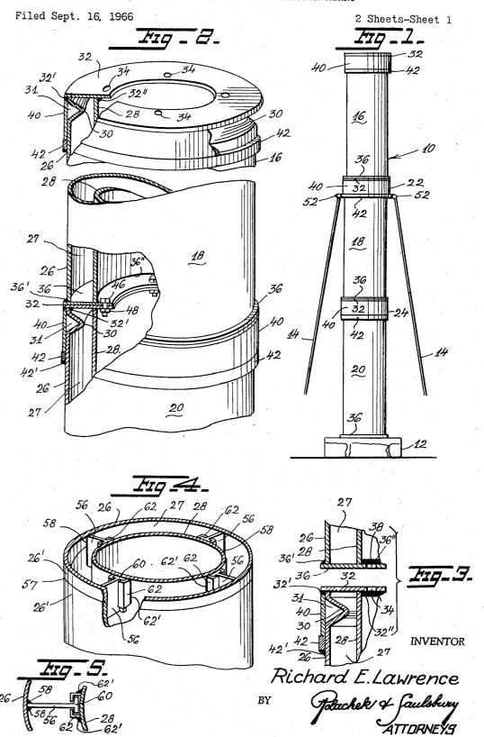
STACK SECTIONS WITH EXPANSION MEANS
