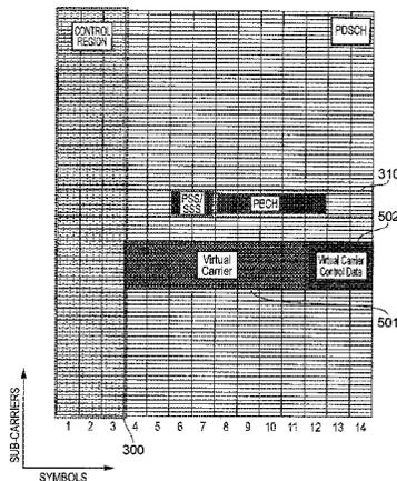
second frequency resources that are used by a host carrier to provide a second set of resource elements, wherein the reduced bandwidth carrier is provided in the first frequency resources in a first sub-frame, wherein the reduced bandwidth carrier is provided in third frequency resources in a second sub-frame after the first sub-frame, and wherein the third frequency resources are within and smaller than the first frequency resources.
