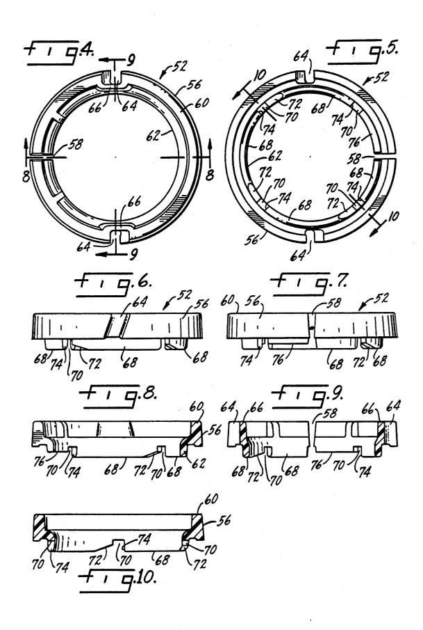
FIG. 6 is a side view of the flow control ring illustrating one of the flow control notches;
