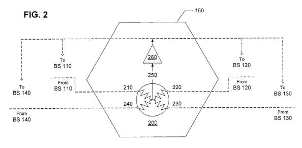
(57) Abstract: A distributed wide area coverage system is disclosed that effectively expands the coverage area of the local wireless links by combining the signals from local area base stations and routing the combined signal back to the base stations. The base stations provide two-way open wireless communication channels among mobile devices situated within wireless signal coverage area of each of the base stations.
