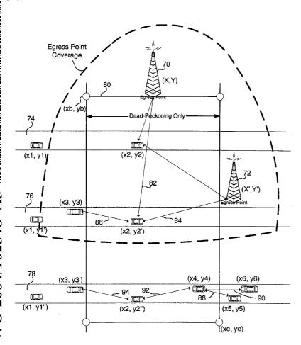
(57) Abstract: An enhanced dead reckoning method determines the position of a participating vehicle (x2, y2'). The participating vehicle is unable to receive signals from global positioning satellites. The position is calculated by way of observed time difference calculations and received signal strength indications. The position is also calculated communicating with other participating vehicles (x3, y3) or egress points (70).
