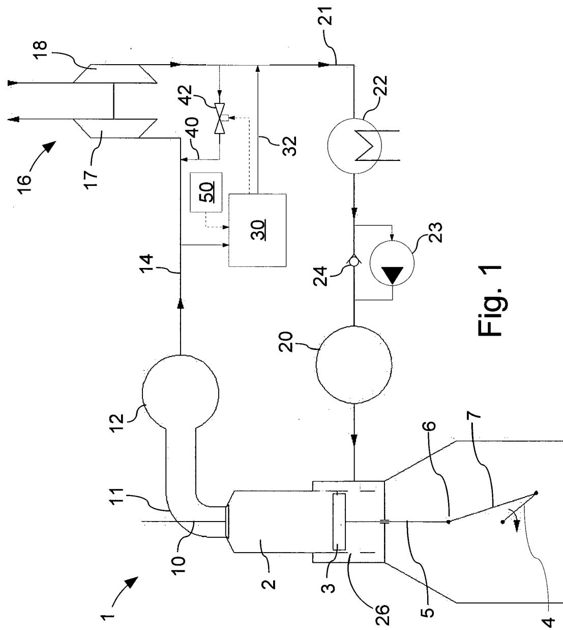
LARGE TURBOCHARGED TWO-STROKE DIESEL ENGINE WITH EXHAUST
