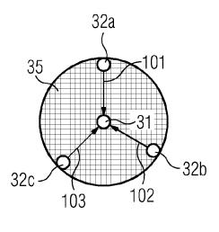
second base coil system, and the third base coil system are arranged such that the mechanical surface stresses of the workpiece can be at least partially determined. A method for determining the mechanical surface stresses is also provided.
