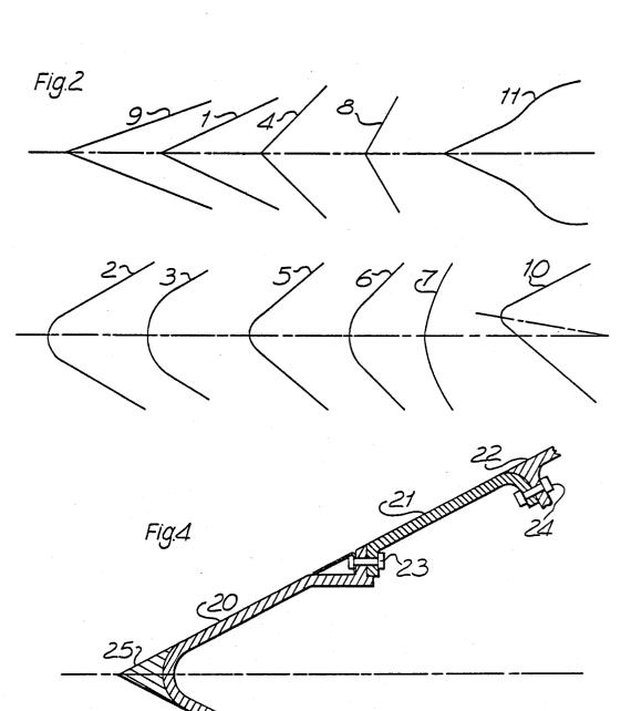
SPINNER SHAPES ICING PROFILES 1–11 INCL. ICE REMAINING AFTER 10 MINUTES AT  $1\cdot0\,\mathrm{gm/M}^3$  –20°C AND TUNNEL NOZZLE VELOCITY OF 300 F.P.S. 8 2000 R.P.M. 88 200 Fig.3 700 WEIGHT OF ICE REMAINING. gm.
