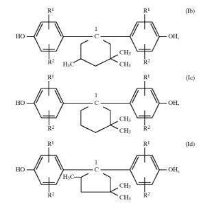
the 1,1-bis(4-hydroxyphenyl)-3,3,5with trimethylcyclohexane (formula Ib having R<sup>1</sup> and R<sup>2</sup> equal to H) being particularly preferred.
