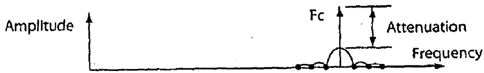
Figure 5c: Excitation Spectrum plus Attenuated Quadrature Modulation
