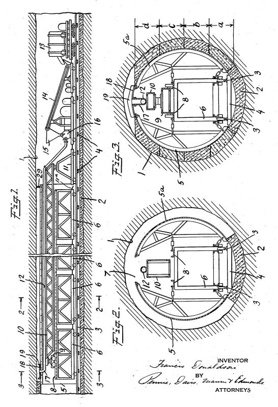
METHOD OF AND APPARATUS FOR CONSTRUCTING CONCRETE TUNNELS
