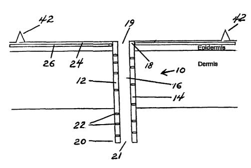
(57) **Abstract:** A device for obtaining a sample of interstitial fluid from a patient for use in monitoring the level of blood glucose in the patient. The device comprises a hollow tube having a wall surrounding a cavity, wherein the wall of the tube contains a multiplicity of pores. The hollow tube is inserted into the tissues through the skin with the help of anintroduction needle. No external suction is applied.
