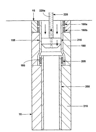
(57) Abstract: Plastically deforming and radially expanding a first tubular member (155) within a wellbore (10) form a mono-diameter wellbore casing. A second tubular member (200) is then plastically deformed and radially expanded, overlapping the first tubular member (155). Then the second tubular (200) and the overlapped portion of the first tubular (155) are expanded.
