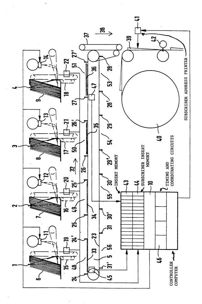
METHOD AND SYSTEM FOR SELECTIVELY COLLATING SUBJECTIVELY DIFFERENT PRINTED COPY PRODUCTS, PARTICULARLY DIFFERENT NEWSPAPER INSERTS FOR TARGETED DISTRIBUTION
