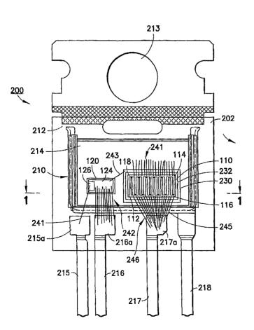
(57) Abstract: A semiconductor device package includes a die pad, a substrate disposed on the die pad, and a III-nitride based semiconductor device disposed on the substrate. The device package may also include a second semiconductor device disposed on the die pad or the substrate, which device may be electrically connected to the III-nitride based device to form a circuit.
