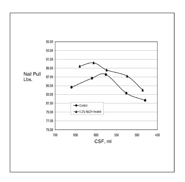
FIG. 6. EFFECT OF 0.2% SODIUM HYDROXIDE TREATMENT ON THE NAIL PULL STRENGTH OF GYPSUM BOARD (NAIL PULL RESULTS WERE NORMALIZED WITH PAPER BASIS WEIGHT)
