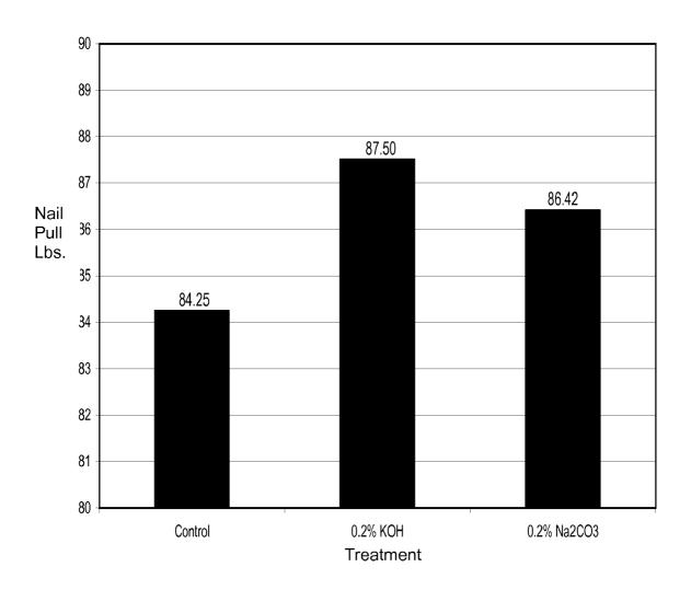
EFFECT OF CATIONIC STARCH ON THE NAIL PULL STRENGTH OF GYPSUM BOARD (NAIL PULL RESULTS WERE NORMALIZED WITH PAPER BASIS WEIGHT)
