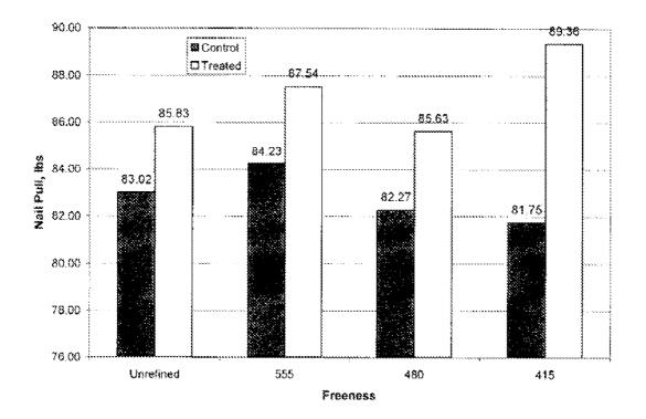
FIG. 3 NAIL PULL STRENGTH OF SMALL BENCH BOARD WITH CAUSTIC TREATED AND UNTREATED FIBERS (NORMALIZED WITH PAPER BASIS WEIGHT)
