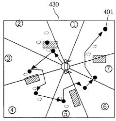
GENERATE OBSTACLE AVOIDANCE PATH PASSING THROUGH AVERAGE POSITIONS
