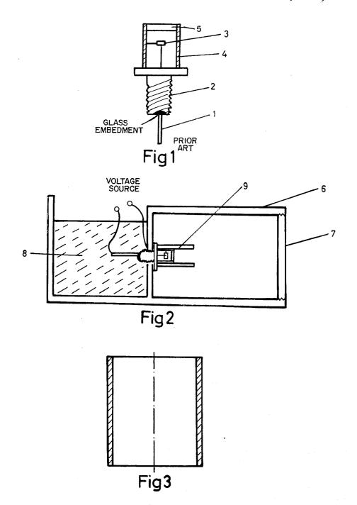
COLD TRAP FOR LASER DIODES
