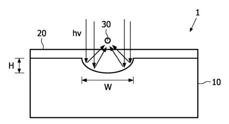
(57) Abstract: The invention relates to a device comprising a first material (10) and a second material. (20) whereby the first and the second material are so provided towards each other as to form at least one focusing microstructure with a focal point (30) located outside of the first material.
