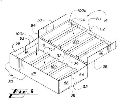
(57) Abstract: A carton (10) includes a composite vertical wall which includes a first wall (22) provided by a panel of a first blank (14) for forming a carton, and a reinforcing member (100b) formed from a second blank (100). The reinforcing member (100) includes at least one substantially vertical rib (104).
