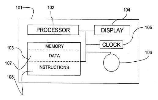
(57) Abstract: A system and method for generating a One Time Password (OTP) based upon a value TEC that can change based both upon the occurrence of an event and the passage of time. The OTP can be computed at a token and sent to a verifier. The verifier stores exact or estimated parameters necessary to compute one or more expected OTPs from the token, including TEC. The value TEC can be synchronized between the token and the verifier.
