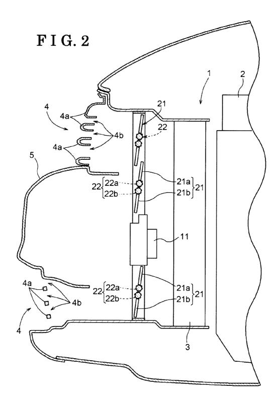
20 Warning lamp -21 Grill control mechanism for vehicle Movable member Control means Electric motor Ambient temperature sensor Cooling medium temperature sensor Speed sensor
