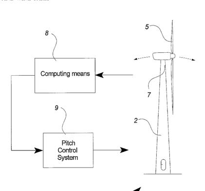
(57) Abstract: The invention relates to a method for controlling a wind turbine connected to the utility grid comprising steps of detecting a fault of the utility grid, and controlling one or more rotor blades in a fault mode wherein said one or more rotor blades are pitched in order to stabilize the rotor speed within an over speed range. The invention also relates to a wind turbine and a wind park comprising at least two wind turbines.
