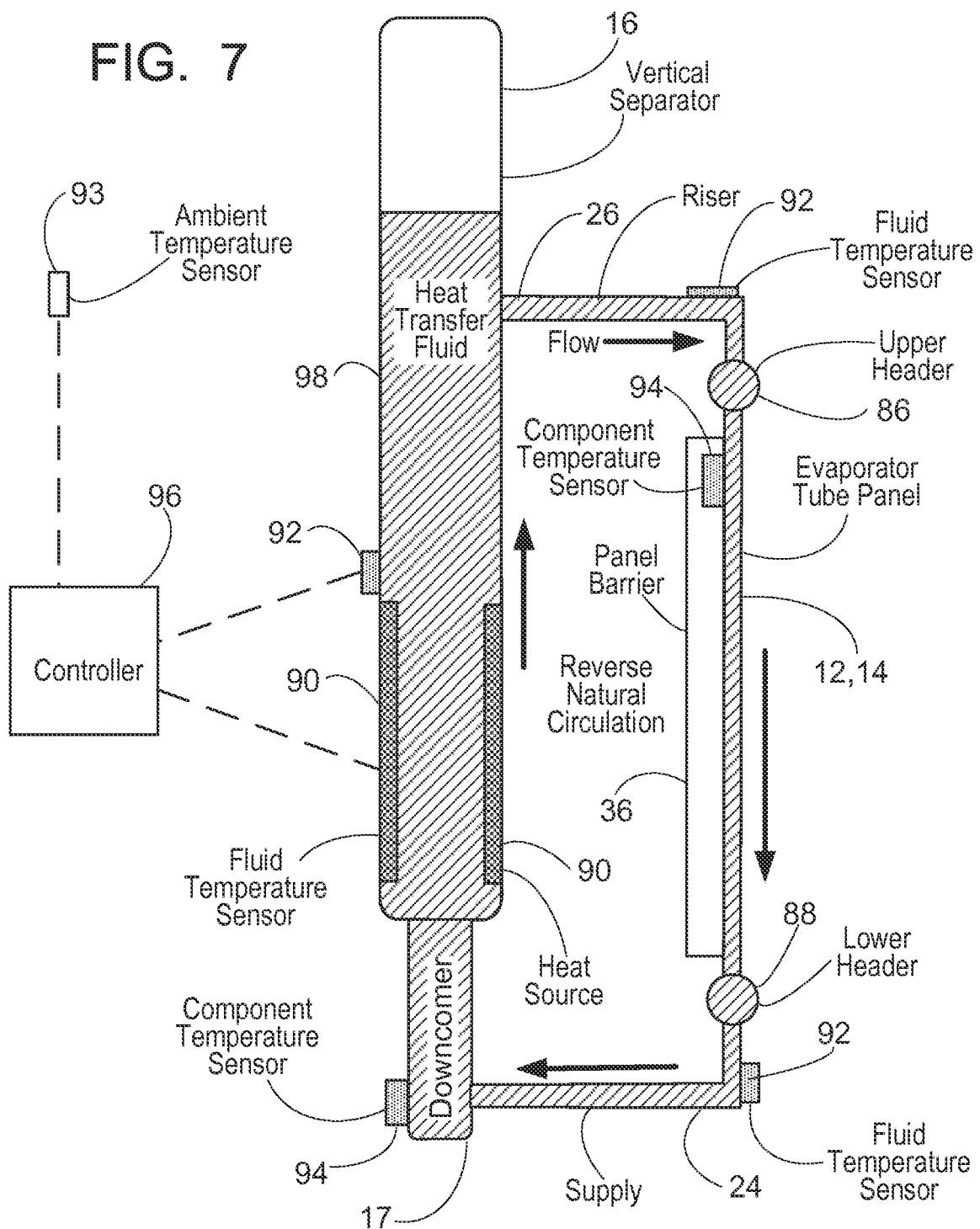
Freeze Protection Via Heat Source Located On
