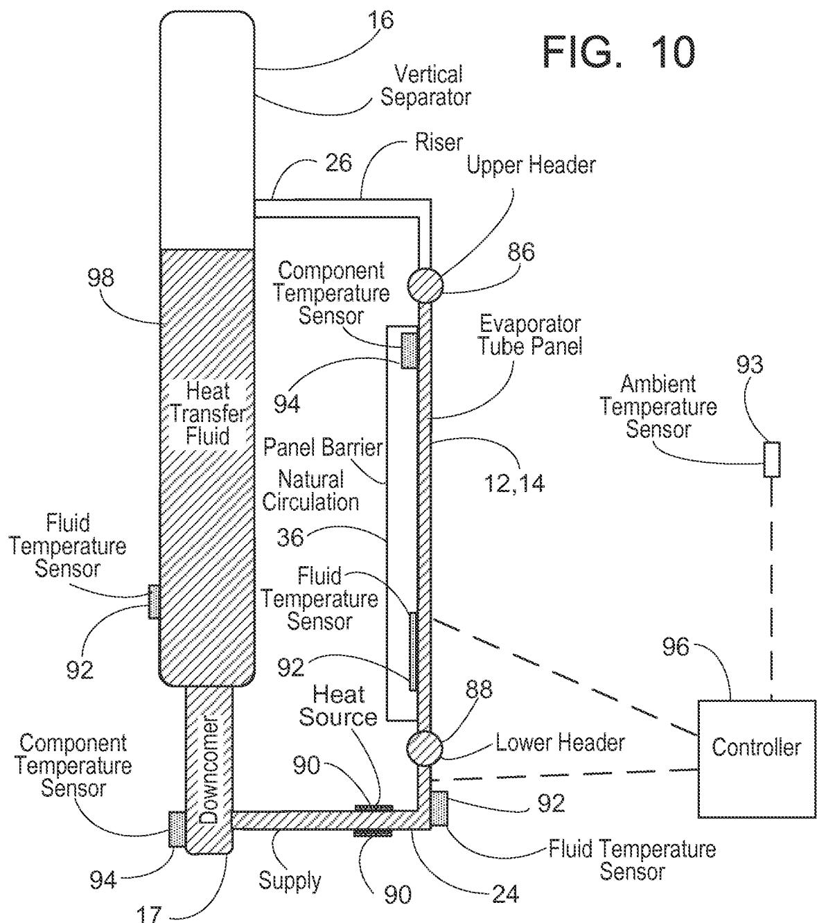
Freeze Protection Via Heat Source Located On
