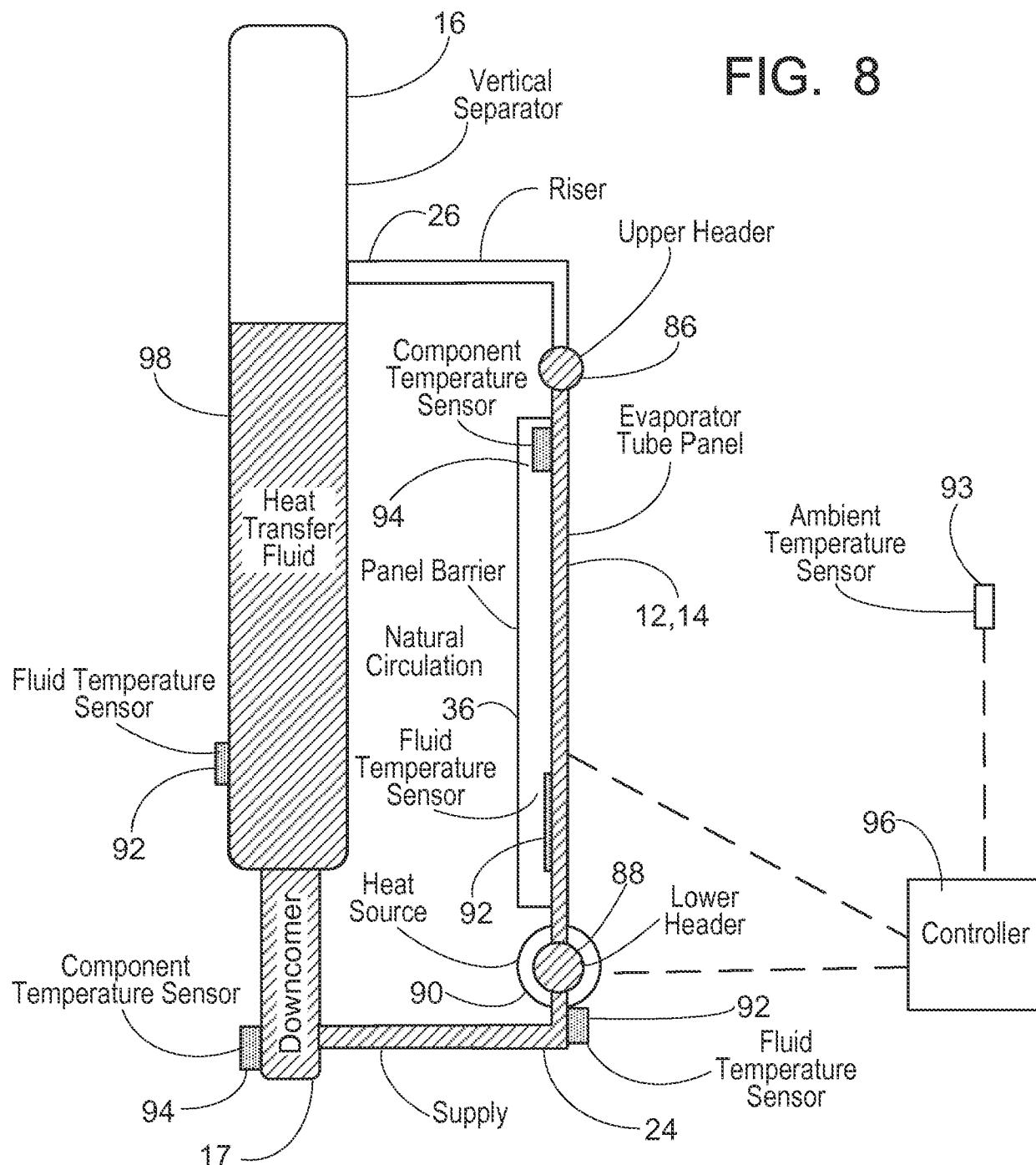
Freeze Protection Via Heat Source Located On
