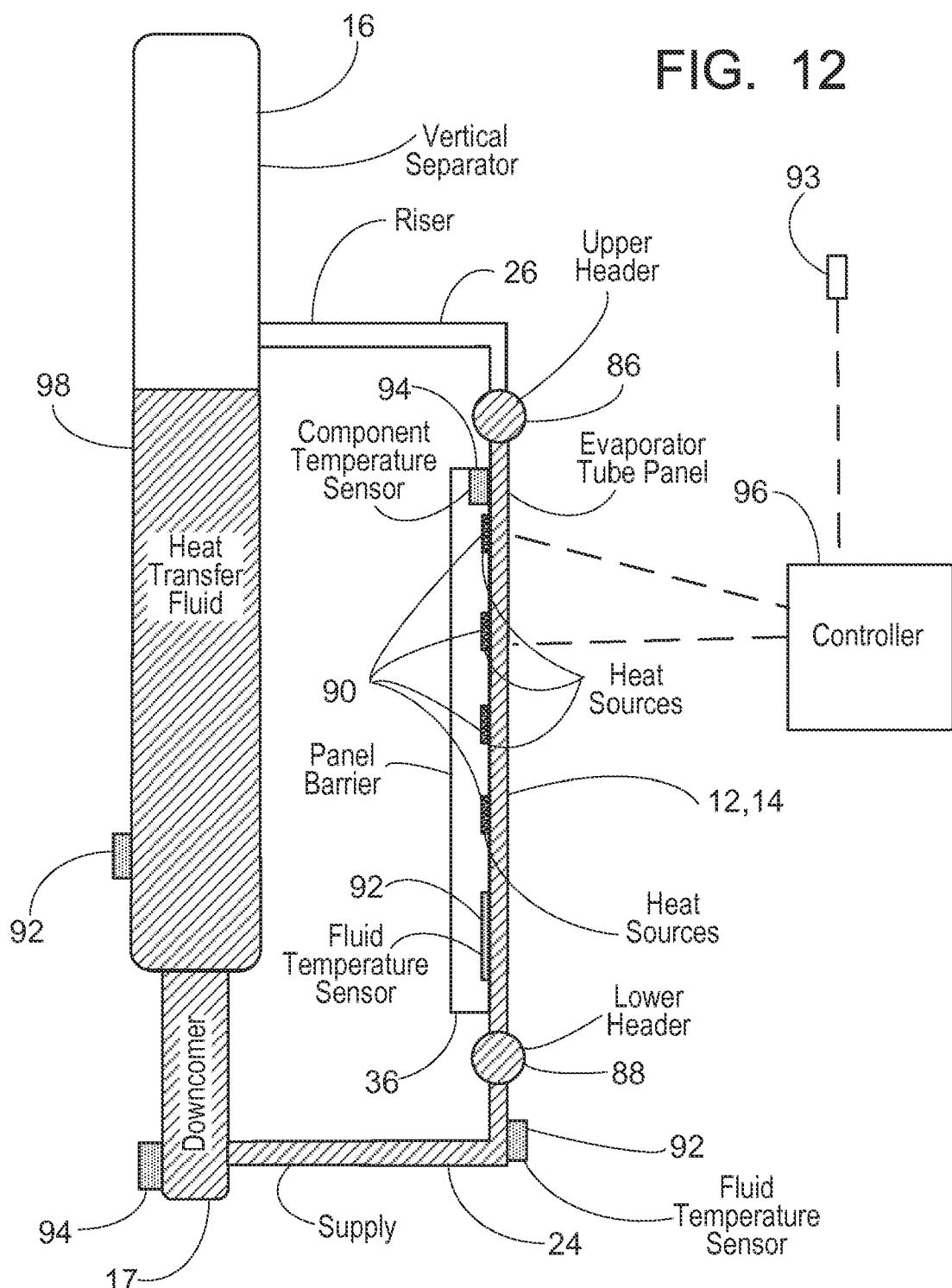
Freeze Protection Via Heat Source in Contact
