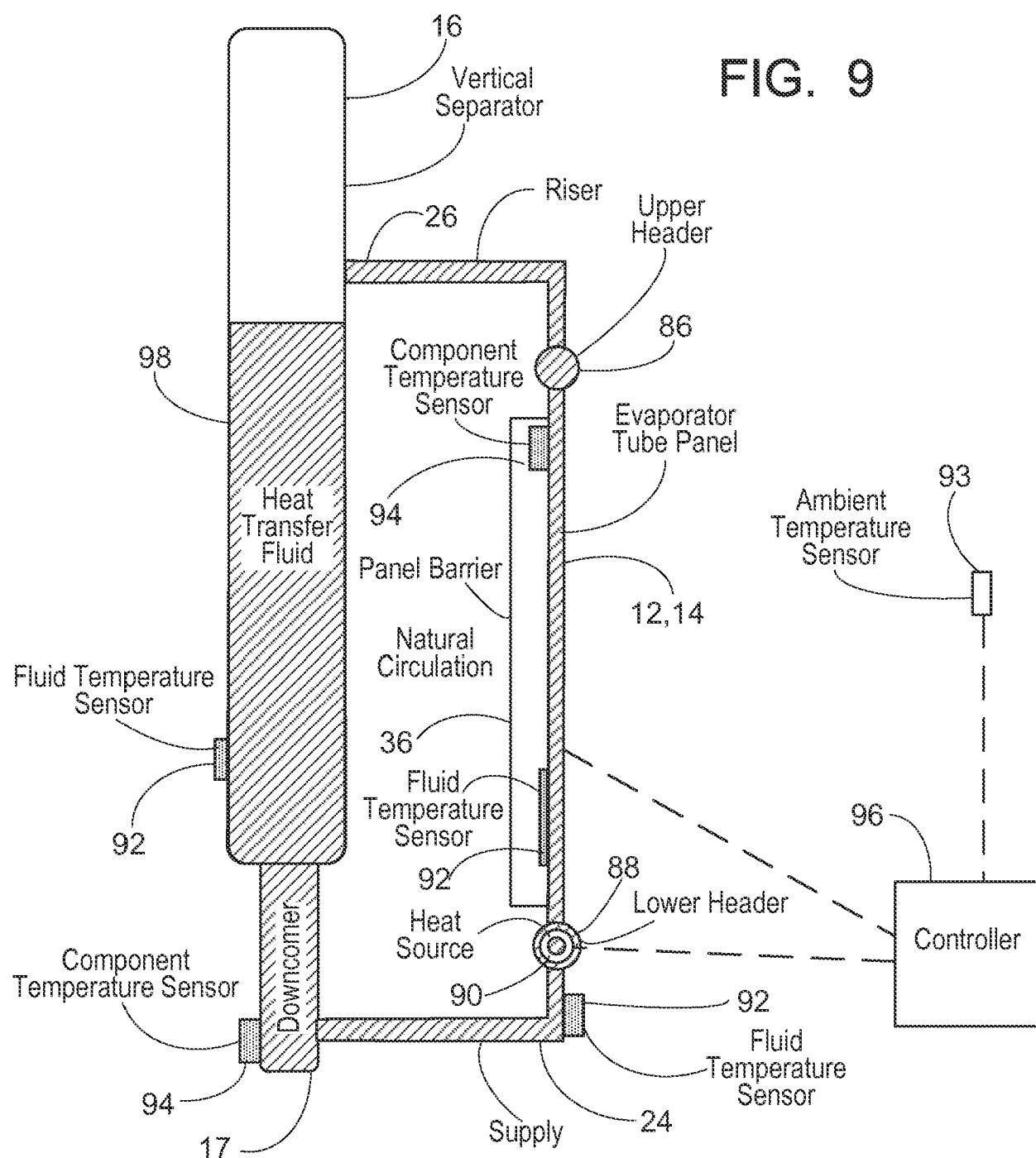
Freeze Protection Via Heat Source Located
