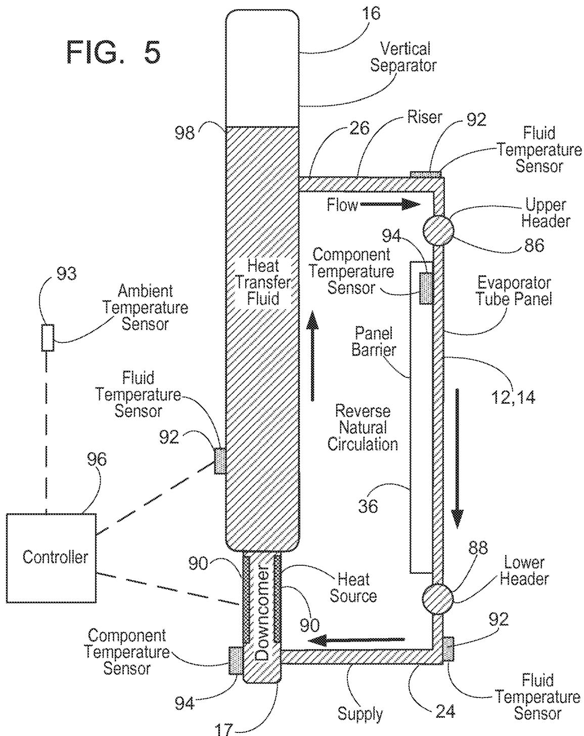
Freeze Protection Via Heat Source Located
