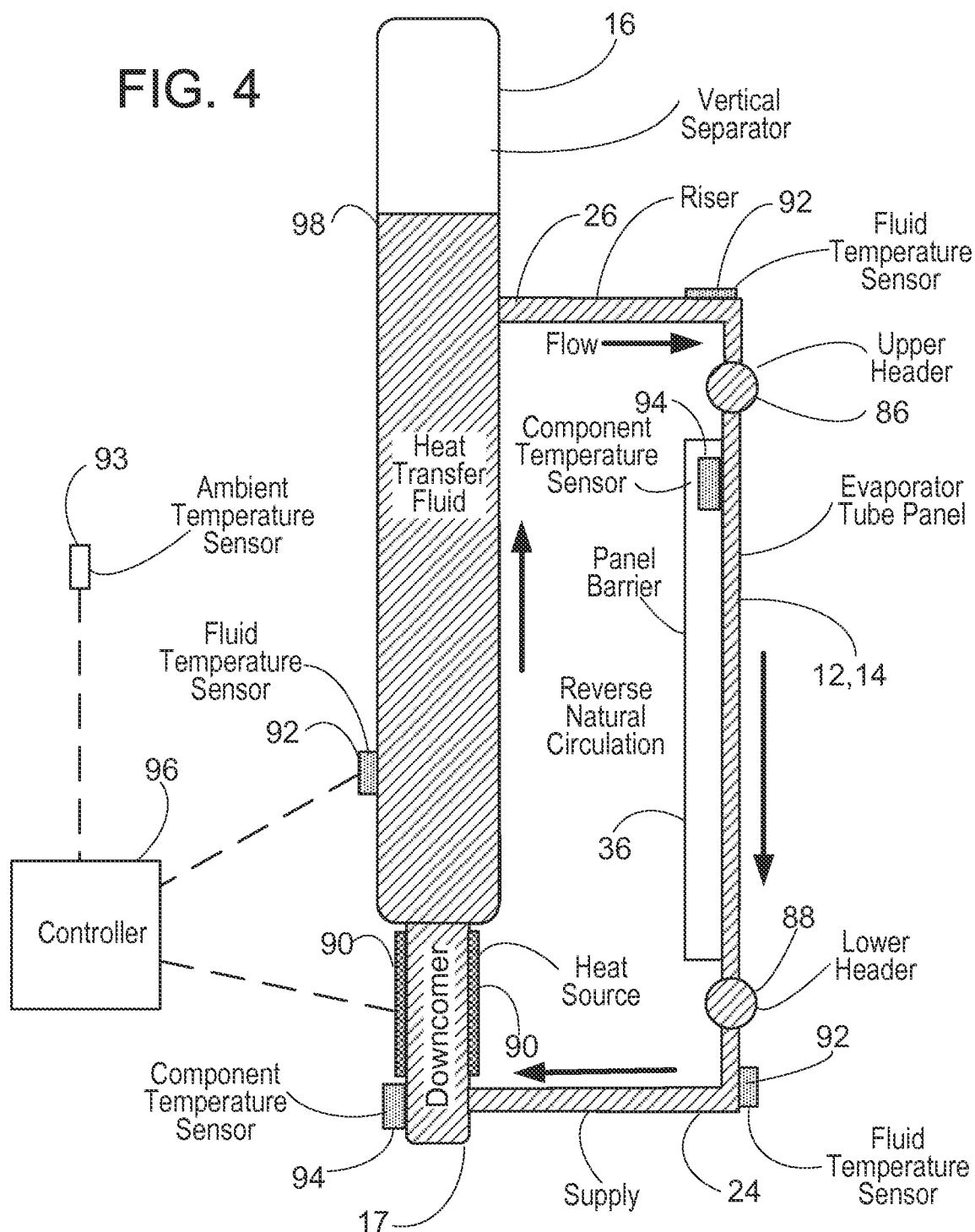
Freeze Protection Via Heat Source Located On
