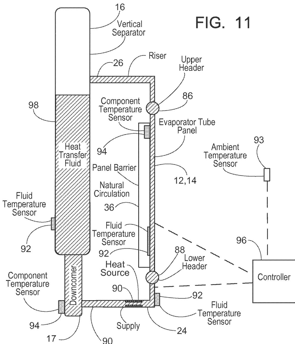
Freeze Protection Via Heat Source Located On
