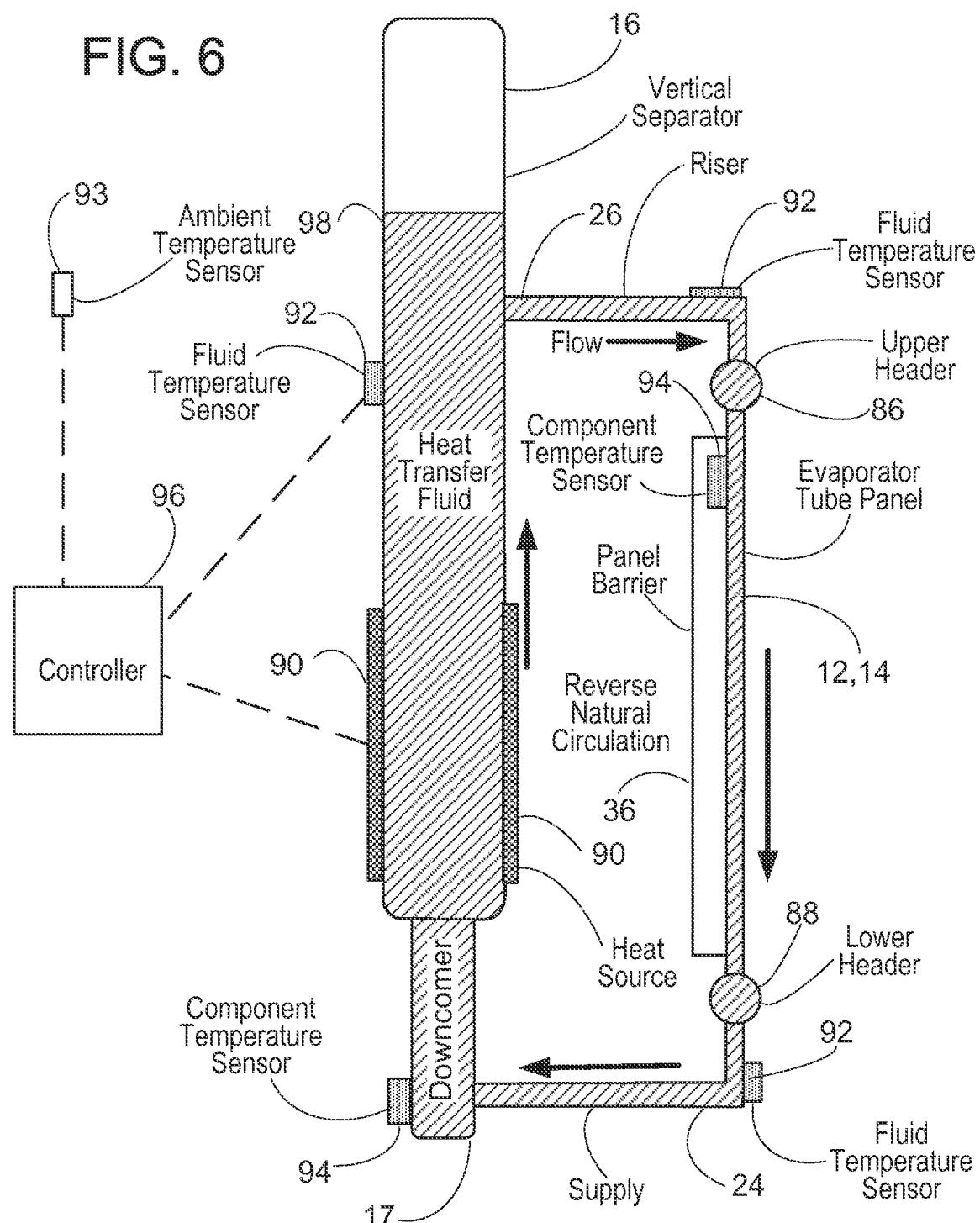
Freeze Protection Via Heat Source Located On
