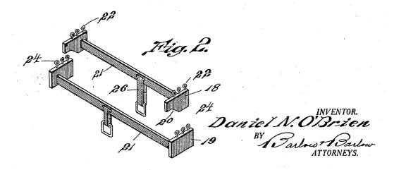
HARNESS MECHANISM FOR A LOOM
