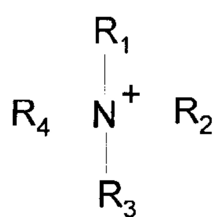
wherein R<sub>1</sub>, R<sub>2</sub>, R<sub>3</sub> and R<sub>4</sub> each independently are a C1-C6 alkyl or a C1-C6 hydroxyalkyl group, and further wherein the cationic group is connected to the starch via an ether or an ester linkage.
