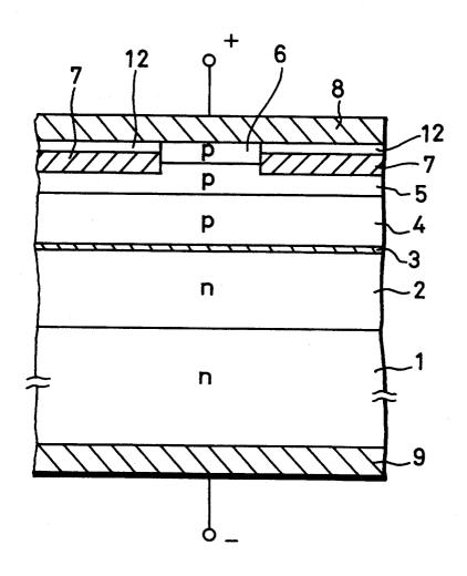
SEMICONDUCTOR LAYER HAVING FIRST AND SECOND CLADDING LAYERS AND AN ACTIVE LAYER FORMED OF A II-VI GROUP COMPOUND AND A CURRENT CONFINEMENT LAYER COMPRISING A METAL OXIDE
