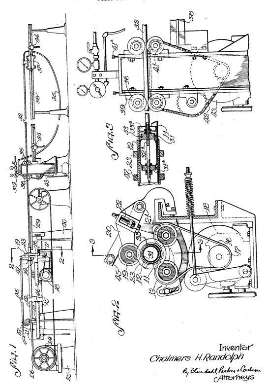
PROCESS OF AND APPARATUS FOR GRINDING INTERNAL SURFACES OF TUBES
