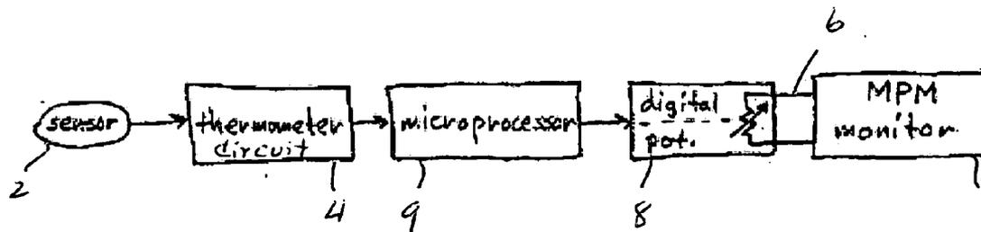
Fig. 3 Dual Thermistor Method
