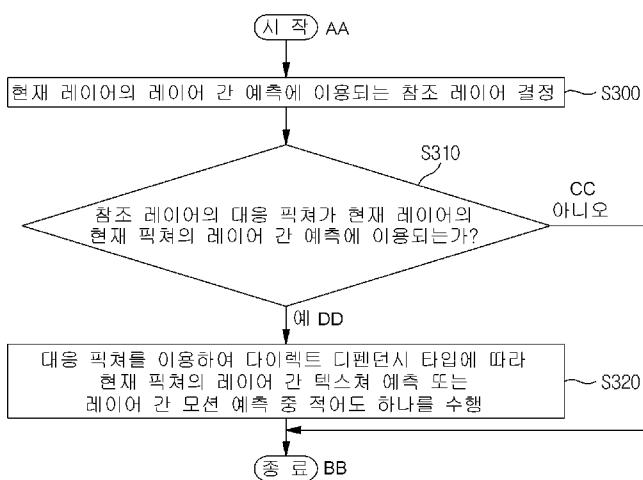
300 ... Determine reference layer used for inter-layer prediction of current layer
