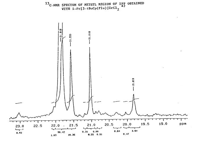
a) 60°C Bulk Polymerization; 1.0 mg iPr[3-tBuCp(Flu)]ZrCl<sub>2</sub>; 5 mL HAO (10 vt% sol.).
