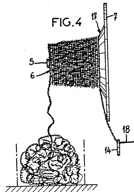
**DEVICE FOR THE RECOVERY AND REMOVAL OF A FALSE SELVEDGE IN A SHUTTLELESS LOOM**
