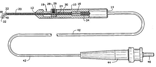
(57) Abstract: A microsurgical laser probe is provided with distal end (12) portion of an optic fiber (42) that projects from a tubular sleeve (20) of the probe and can be caused to bend relative to the probe sleeve by manual manipulation of a mechanism (26) on a handle of the probe.
