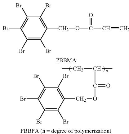
[0003] In its most general form, the route of synthesis of pentabromobenzyl acrylate is based on the reaction between pentabromobenzyl halide (i.e., chloride or bromide) with a salt of acrylic acid, e.g., sodium acrylate.
