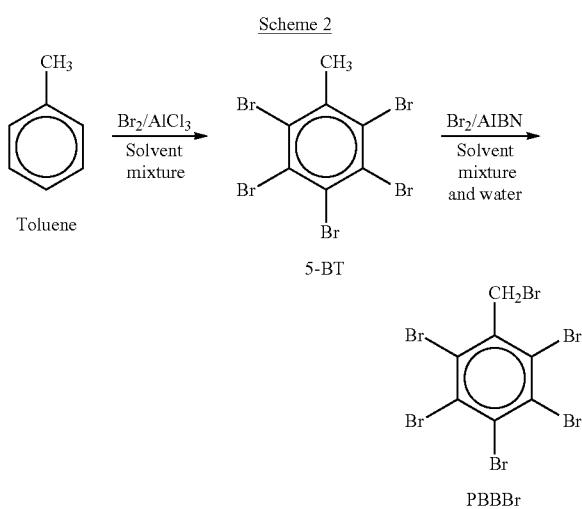
**[0024]** The radical bromination reaction of pentabromotoluene is carried out in the presence of a suitable catalyst, such as 2,2-azodi-isobutyronitrile (AIBN), as illustrated in Example 5 of U.S. Pat. No. 6,028,156. However, it has now been found that dibenzoyl peroxide (DBP) can be used instead of AIBN as a catalyst in the bromination reaction of pentabromotoluene to give high purity pentabromobenzyl bromide (e.g., of not less than 99.3%, as indicated by HPLC analysis).
