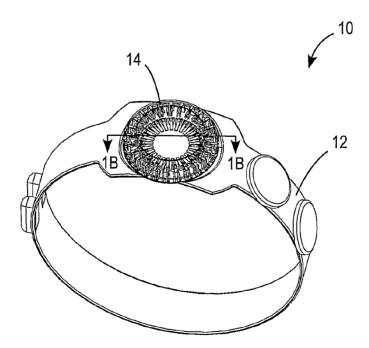
(57) Abstract: An arrangement comprises a housing containing one or more components configured for at least one of body fluid sampling and analysis. The arrangement includes a housing containing one or more components configured for at least one of body fluid sampling and analysis, and a body attachment element. The housing and the body attachment element are connected by a quick-release mechanism configured to facilitate removal of the housing from the body attachment element.
