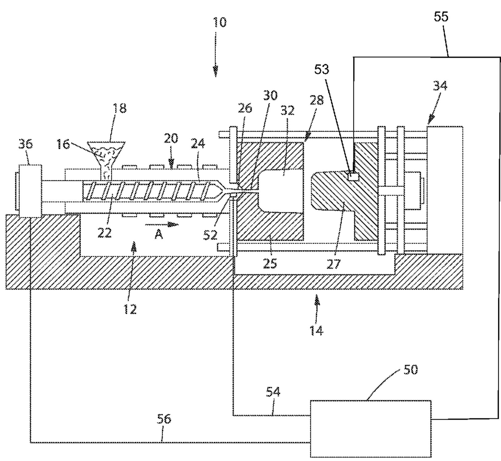
(57) Abstract: A method and a machine that account for changes in material properties of molten plastic material during an injection run. If viscosity of the molten plastic material changes during an injection run, a controller alters a step time of the injection cycle to ensure that molten plastic material completely fills and packs a mold cavity to prevent part flaws such as short shots or flashing.
