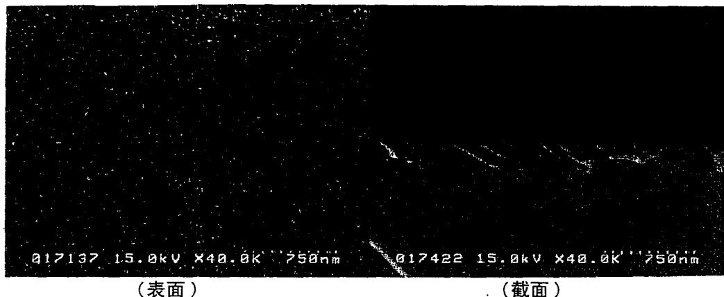
**B** $O_2/(Ar+O_2)=0\%$ , 厚度 500nm
