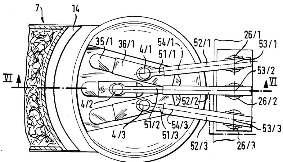
**ELECTRIC ARC FURNACE HAVING A SPACE PROVIDED ON ONE SIDE OF THE FURNACE VESSEL FOR ACCOMMODATING CHARGING MATERIAL**
