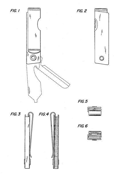
FIG. 1 is a view of one side of a combination knife and money clip embodying my new design with the blades being shown in dotted lines in the extended position;
