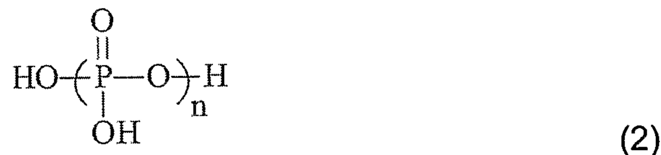
where n is 1 to 12 or higher. Note, under this structure, when n is 1, it is monomeric phosphoric acid. It is believed that when n is greater than 1, 20 due to its polymeric nature, PPA in the filament 12 is strongly associated with the polybenzazole (PBZ), and its removal or extraction during the washing step(s) is much more difficult than washing out monomeric phosphoric acid.
