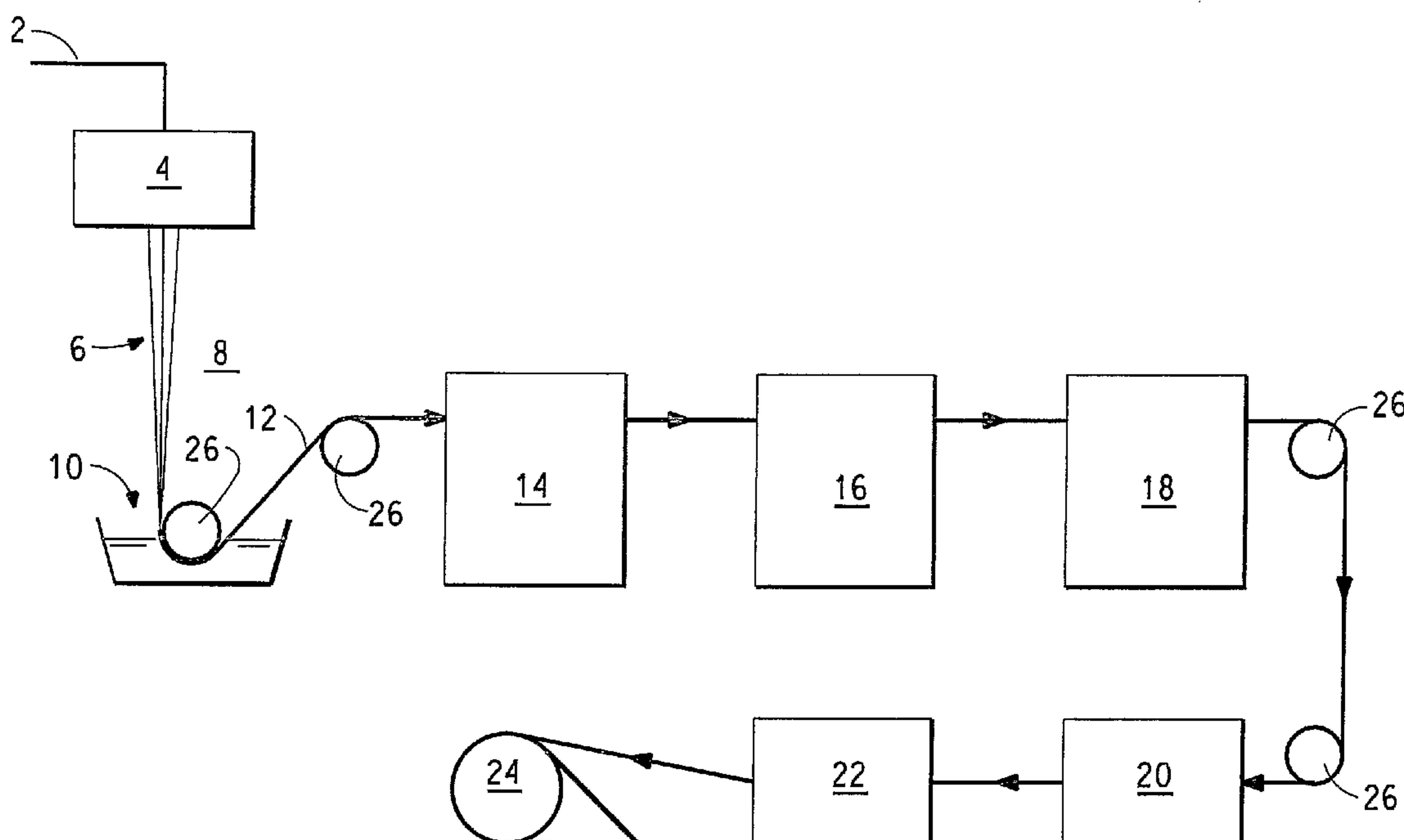
(57) Abstract: The present invention relates to polybenzazole (PBZ) fibers and processes for removing polyphosphoric acid from a polybenzazole dope filament. The invention further relates to yarns, fabrics, and articles incorporating fibers of this invention, and processes for making such yarns, fabrics, and articles.
