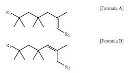
wherein  $R_1$  is a polyisobutylene chain with a number average molecular weight of about 200 to about 5000 Daltons; and  $R_2$  is a carboxyl-containing group.
