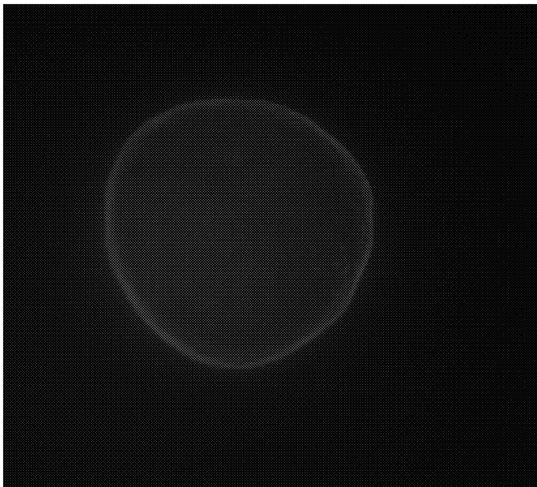
Epifluorescent microscopic images of a microcapsule containing FITC-labeled lysozyme in PBS. The imaged microcapsule is approximately 7 micrometers in size.
