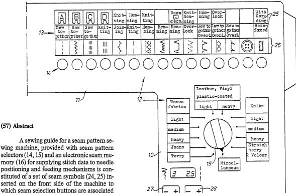
Associated circuits in the electronics control the indicating means at the symbols, whereby some are indicated as suitable for the sort of cloth pointed out by the switching means. The seam selection is then effected by actuating the button of the selected symbol. The electronics comprise circuits for supplying ideal data controlling stitch length and stitch width for the selected cloth and seam, respectively.
