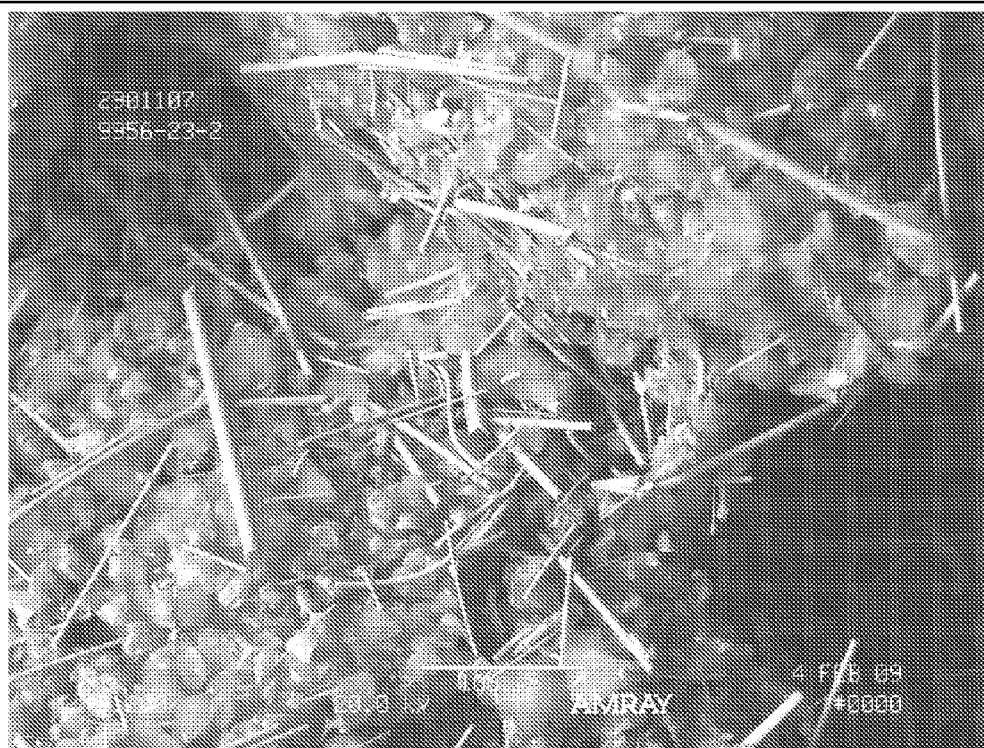
Figure 3: Scanning electron micrograph of an aerogel - mineral fibre composite made with high pH water.
