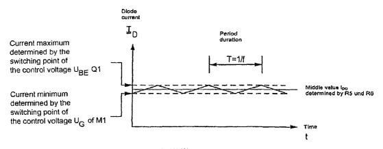
Frequency: f < 100 kHz (determined by  $U_{\rm NETZ}$  and suitable dimensioning of L1 and the switching thresholds for the control voltages  $U_{\rm SR}$  and  $U_{\rm O}$  of the power transistors Q1 and M1)
