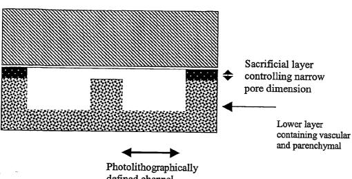
defined channel dimension - resolution limit is 25x higher than vertical pore
