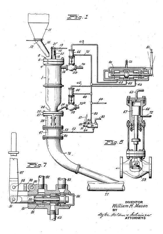
PROCESS AND APPARATUS FOR DISINTEGRATION OF FIBROUS MATERIAL
