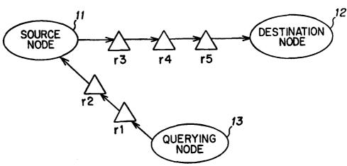
hop router from the IP routing table. If this fails, the method reverts to the incrementing TTL mechanism.
