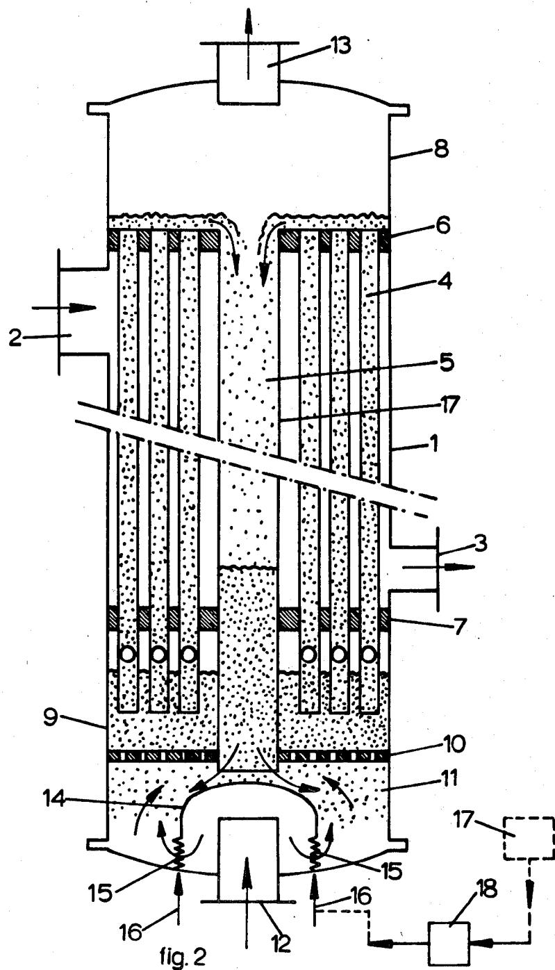
**APPARATUS FOR USE IN CARRYING OUT A PHYSICAL AND/OR CHEMICAL PROCESS, FOR EXAMPLE A HEAT EXCHANGER**
